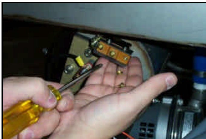
Removing the thermostat screws.
